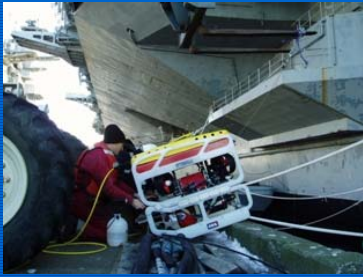
Falcon DR with IMU preparing to launch for inspection under mothballed aircraft carrier.
