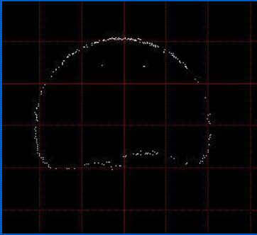
Figure 1: x,y points from scan of pipeline showing sedimentation.
