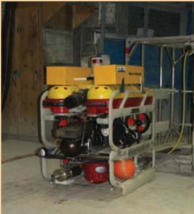
The SAAB SeaEye Falcon DR , outfitted for deployment in the Cigar Lake Mine. Note the SoundMetrics DIDSON sonar mounted below the primary camera, the additional DSPL Lights on the starboard side of the ROV, and the Teledyne-RDI DVL on the instrument skid. Also note the additional syntactic foam installed on the Falcon to maintain neutral buoyancy. The Outland Pan/Tilt cameras were installed immediately after this picture was taken.
