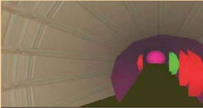
A view from the perspective of the Falcon, from within the Shaft 1 chamber alongside the elevator that carried the deployment garage to the 480-meter level. SeaVision color-coded the different spurs off of the primary drift so that the SeaView's ROV operator knew which tunnel was the target. The spur tunnels do not actually come into the interior of the main drift; rather, that is an artifact of the 3DTV shapes used to develop the concept model for the project.
