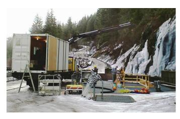
face power supply system, umbilical distance counter, 3 video cameras (typically one low light color on 180° tilt platform and 2 fixed cameras) and a range of profiling and imaging sonars, the overall package represents a world class solution to long distance pipeline and tunnel inspections.
