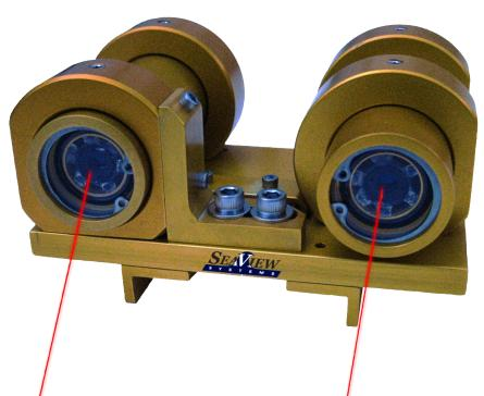
Parallel \$caling Lasers are mounted on top of the center camera and are calibrated so that their parallel beams lie 3"/75mm apart. They point two spots on the subject which can be used for scaling purposes.
