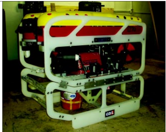
Seeye Falcon DR equipped with an under slung survey skid. The survey skid was custom designed to accommodate the CDL MiniPos Inertial Navigation System as well as a RDI Doppler sonar. Other equipment included a 360 degree scanning profiling sonar and a forward looking obstacle avoidance sonar.
