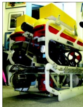
Seavey Falcon DR configured for operation in the Cigar Lake mine. Note CDL minipos and RDI Doppler sonar mounted on survey skid. Also on skid are two Outland Technologies Pan and Tilt cameras and CDL Minipulse profiling sonar. Mounted directly below the center camera is a Didson Multibeam imaging sonar on a platform mechanically slaved to the center camera. Note additional syntactic foam blocks fitted to maintain neutral buoyancy.
