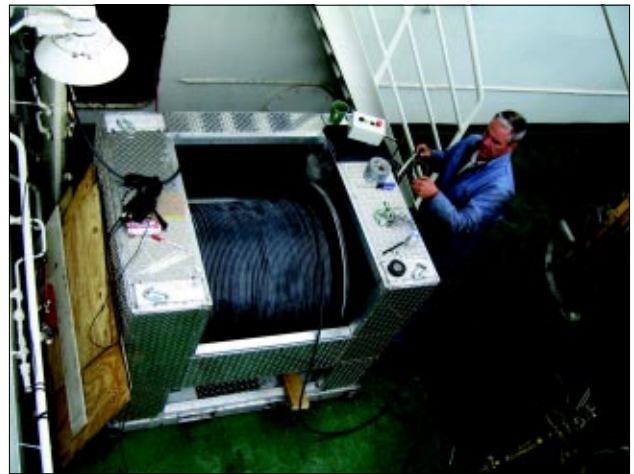
Air freight-able lifting umbilical winch fitted with 4200ft of Kevlar reinforced umbilical cable. Photo also shows 24" sheave wheel which when fitted with a strain sensor provides feedback to winch control processor to provide heave compensation capability.
