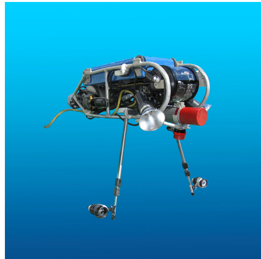
Initial use of the ROV Backbone was to provide auxiliary thrust to SeaBotix LBV150s along with auxiliary lighting and sonar telemetry.
