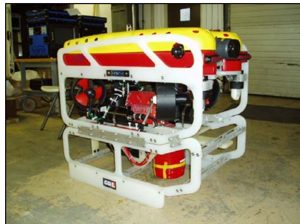
The SeaEye Falcon DR, fitted with an instrument skid that has the CDL MiniPos INS and RD Instruments Workhorse DVL mounted. The calibration routine is actually performed with the skid separate from the ROV, towed from a survey vessel, so that a variety of velocity changes, angular accelerations, and turns can be performed quickly in order to train the Kalman filtering algorithms in the INS.
