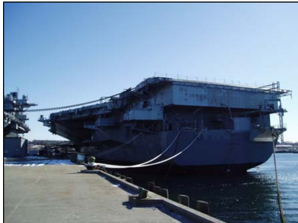
The stern of the decommissioned aircraft carrier USS Forrestal at Naval Station Newport, RI. The mooring lines and chains for the long-term heavy-weather mooring configuration, and the hull itself, prevent survey of the bottom underneath the footprint of the carrier by a vessel.
