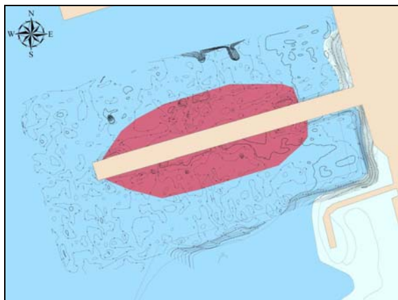
The total hydrographic survey at Pier 1, Naval Station Newport, was used to develop 1-ft elevation contours in the berths surrounding the pier. The area in red represents the footprints in both berths where data collected with the ROV (armed with an aided INS and profiling sonar) completed the restricted-access portion of the survey.
