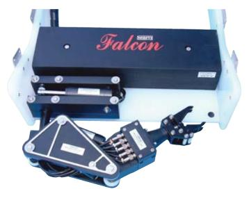
The unique 5 function manipulator arrangement gives excellent dexterity for a small arm and greatly enhances the operational capability of SeaView's Falcon DR ROV. It is ideally suited to retrieval and salvage work as well as sample collection.
