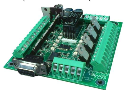
Power efficiency is important in remote data collection systems that are typically solar-powered. Systems such as the Real-time Coastal Observation Network (ReCON) require controlling power to sensors and components with currents of up to 2 amps and voltages up to 48 volts. Though there are some off-the-shelf solutions available, these systems either consume unnecessary power, or are limited in the amount of current and voltage that they can handle.
