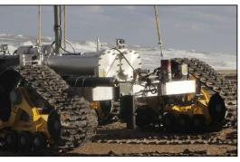
(Top) SurfROVer emerges from heavy surf conditions during field trials at the ocean-side shoreline at Duck, North Carolina. In this configuration, targeting relatively shallow water, the mast supports a GPS antenna that allows precise navigation control and location of survey data. (Bottom) The front view of SurfROVer shows a host of survey equipment, including lights, HD and SD cameras, multiple sonar imagers and a current profiler.
