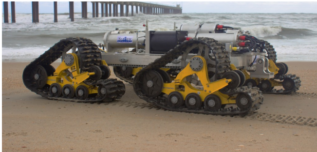
Fig. X. SeaView's SurfROver towing White River Technologies' EM sensor array in the surf at the Army Corps of Engineers facility at Duck North Carolina.
