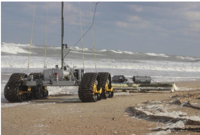
Fig. 3. Configuration of SurfROVer with towed EM sensor array. The blue dot at the center of the vehicle is the location of the GPS mast. An encoder at the tow point was used to monitor the angle of the sensor array relative to the vehicle orientation.
