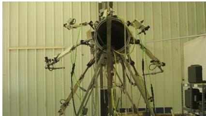
In addition to HD video, Titan can also incorporate profiling sonar to measure the internal surfaces of the tunnel including sediment depth and its payload can be configurable with other specialty sensor suites depending on the particular application requirements.
