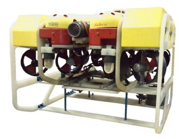
Rather than design and build a new vehicle from scratch, SeaView chose to expand on the many excellent design features of the proven Seaeye Falcon DR. By leveraging our in-house underwater systems engineering resources and our extensive experience operating and maintaining this particular ROV
