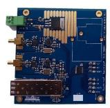
The HD-SDI converter may be stacked neatly on top of SeaView's other optical data cards; the fiber multiplexer and the Gbit Ethernet card. All data may be combined onto a single fiber via a compact wave division multiplexer (CWDM).
