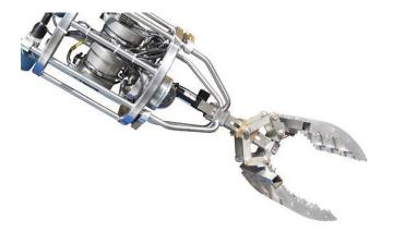
The Smart Grapple is suspended by a heavy lifting line which also controls its vertical motion. The later motion is provided by four vector configured thrusters. It has high intensity, dimmable LED lighting, a pan/orbit/zoom camera as well as a tooling camera integrated into the jaws.
