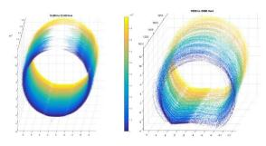
3D point clouds of tunnel interior can be generated from the profiling sonar data. The diagram on the left shows a section of clean tunnel while the diagram on the right has accumulated debris in the tunnel invert. Volumes of sediment can then be calculated from the data.
