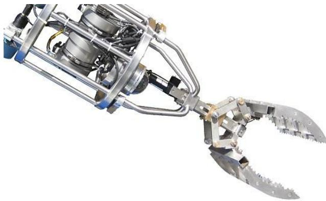
The Smart Grapple is suspended by a heavy lifting line which also controls its vertical motion. The lateral motion is provided by four vector configured thrusters. It has high intensity, dimmable LED lighting, a pan/orbit/zoom camera as well as a tooling camera integrated into the jaws.
