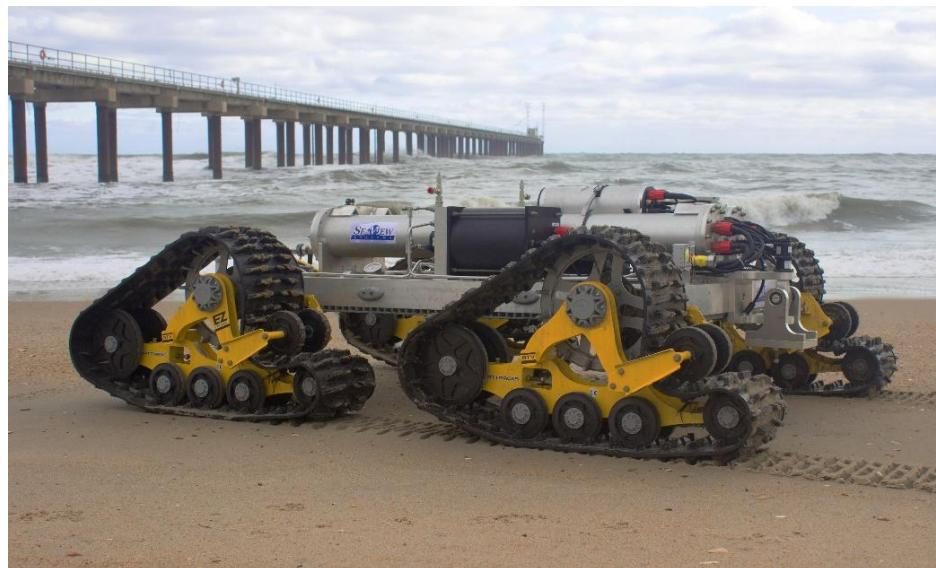
The low-profile design and wide footprint create an extremely stable vehicle for high energy environments and provides an excellent platform for deployment of a cable/pipeline tracker.
