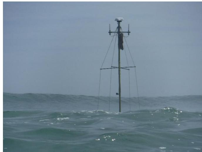
SurfROVer can be controlled via unpowered fiber umbilical or RF (with mast mounted antenna or antenna float system). Position monitoring can be achieved with either on-vehicle GPS (with mast, restricted to lower surf conditions and depths to 6 meters) or available INS capable of accuracies to 0.1 meter.
