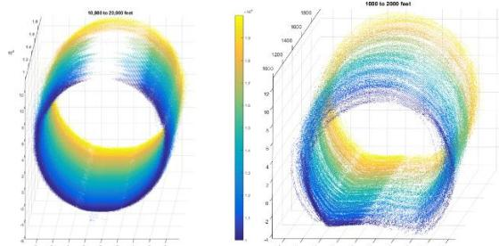
3D point clouds of tunnel interior can be generated from the profiling sonar data. The diagram on the left shows a section of clean tunnel while the diagram on the right has accumulated debris in the tunnel invert. Volumes of sediment can then be calculated from the data.
