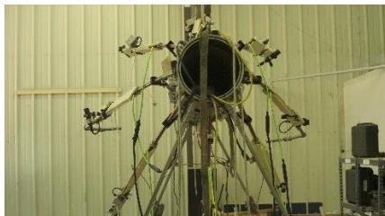
In addition to HD video, Titan can also incorporate profiling sonar to measure the internal surfaces of the tunnel including sediment depth and its payload can be configurable with other specialty sensor suites depending on the particular application requirements.
